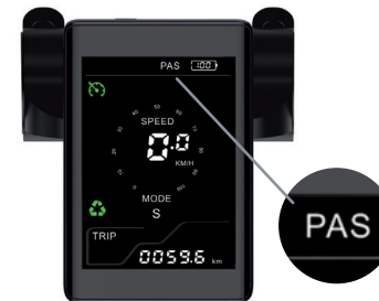
The scooter is in assisted start mode, which means you need to pick up some speed at the start to activate the throttle.
